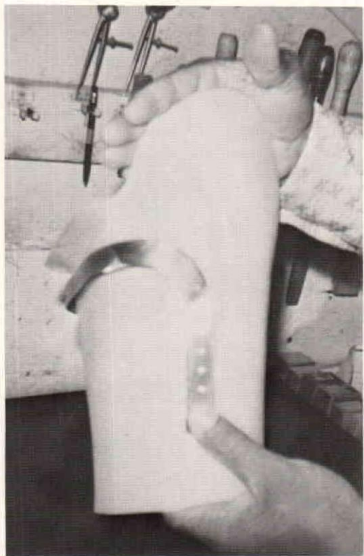
Fig. 9. Lateral view of socket with inverted "U-type" reinforcement piece.
