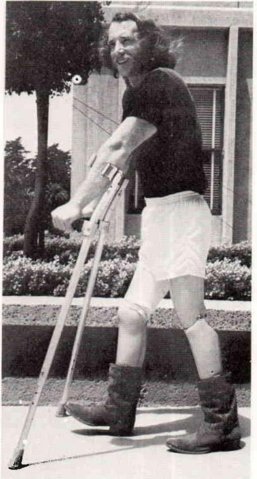
Fig. 20. Case No. 4. Above-knee and below-knee amputee wearing a PTS-AC prosthesis.
