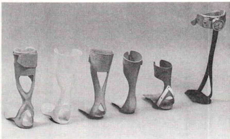
FIG. 1 Various stages of the development and evolution of the TIRR Polypropylene Orthosis. The device on the extreme right is the first approach taken; the one on the extreme left is one version of the latest design.
