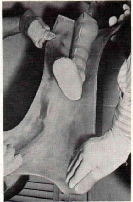
Fig. 7 Placement of Molten Polypropylene Sheet Over Model.
