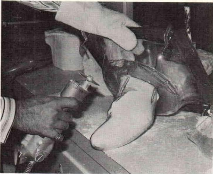
Use a cast cutter to remove most of the material proximal to the trim line of the socket.
