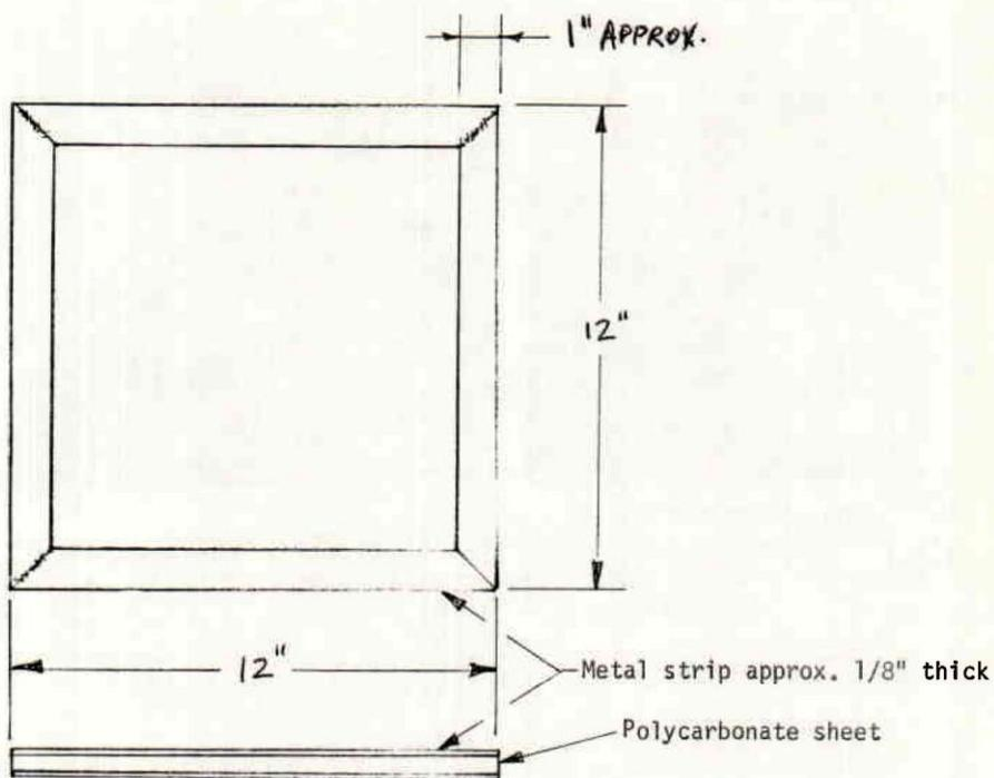
To permit proper handling of the polycarbonate sheet when heated, it is necessary to hold it in simple metal frames. Strip metal about  $\frac{1}{8}$ -in. thick and inexpensive "C" clamps were used in the development program.
