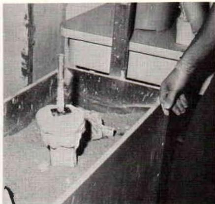
Take a cast of the stump in the usual manner. Pour a male model, using a mandrel to provide the cavity necessary for passage of air during the molding process, and modify as desired. Vaseline or some other parting agent such as "Slipicone" is used on the mandrel. Ordinary plaster-of-Paris may be used, but it is better to use a plaster type that can be heated to 500°F without fracturing.<sup>4</sup>
