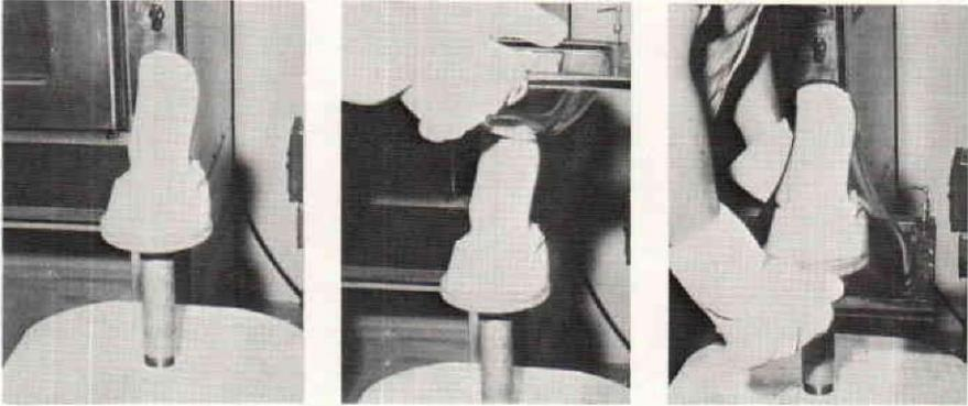
Place the heated male model on the stand. Drape the material still in the frame over the male model, push downward until the polycarbonate contacts the plywood base supporting the male model, and apply 27" Hg vacuum. (Even better results seem to be obtained when the frame and material are turned 180° about the horizontal axis, eliminating the invagination process. It is felt that there is less tendency for formation of built-in stresses when this procedure is used.)
