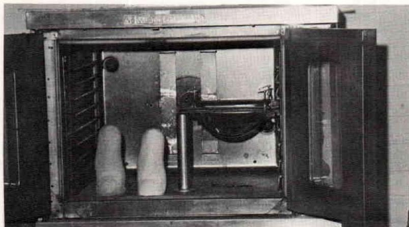
Elevate the temperature to 400 deg. F. until the sheet sags under its own weight to a depth equal to about  $\frac{2}{3}$  the length of the male model. This requires about 10-15 minutes. It is desirable to use another preheated oven. The male model is placed in the 400 deg. F. oven at the same time or slightly before the polycarbonate sheet. A heated model allows the prosthetist more time in forming the socket.
