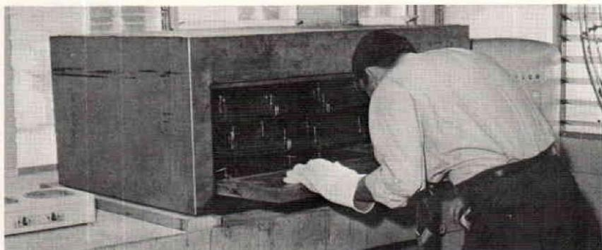
Heat the  $\frac{3}{8}$ -in. material for 36 hours at 275-300 deg. F. to drive out the moisture absorbed by the polycarbonate. If the water is not removed the resulting socket will contain bubbles. It must be maintained at a temperature well below the melting point. A pizza oven was used quite satisfactorily in the development program.
