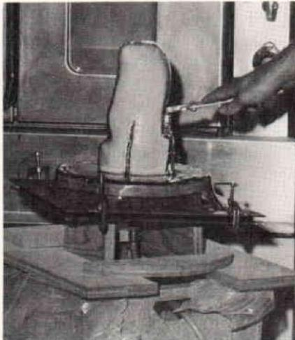
A sheet of polycarbonate up to  $\frac{3}{8}$ -in. thick, after being dried and heated properly, is simply pulled over a male model of the stump and drawn into place with a vacuum supply. No special tooling is required, and no extra care is required to obtain satisfactory results. The socket can be worked with ordinary tools, can be bonded readily, and is sufficiently strong for use in most prosthetics applications. Some of the properties of polycarbonate sheet are given in Appendix A.
