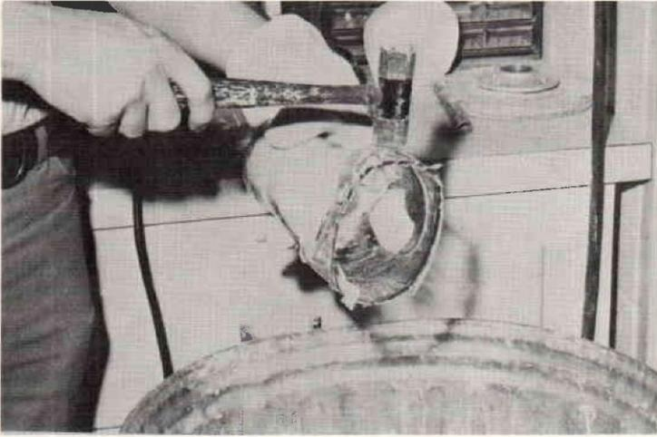
When the socket has cooled to the point where it can be handled easily, remove it and the cast from stand (this is only a matter of minutes). Remove the plaster, usually by knocking on the outside of the socket with a rubber hammer. The larger the mandrel used, the easier this step is.
