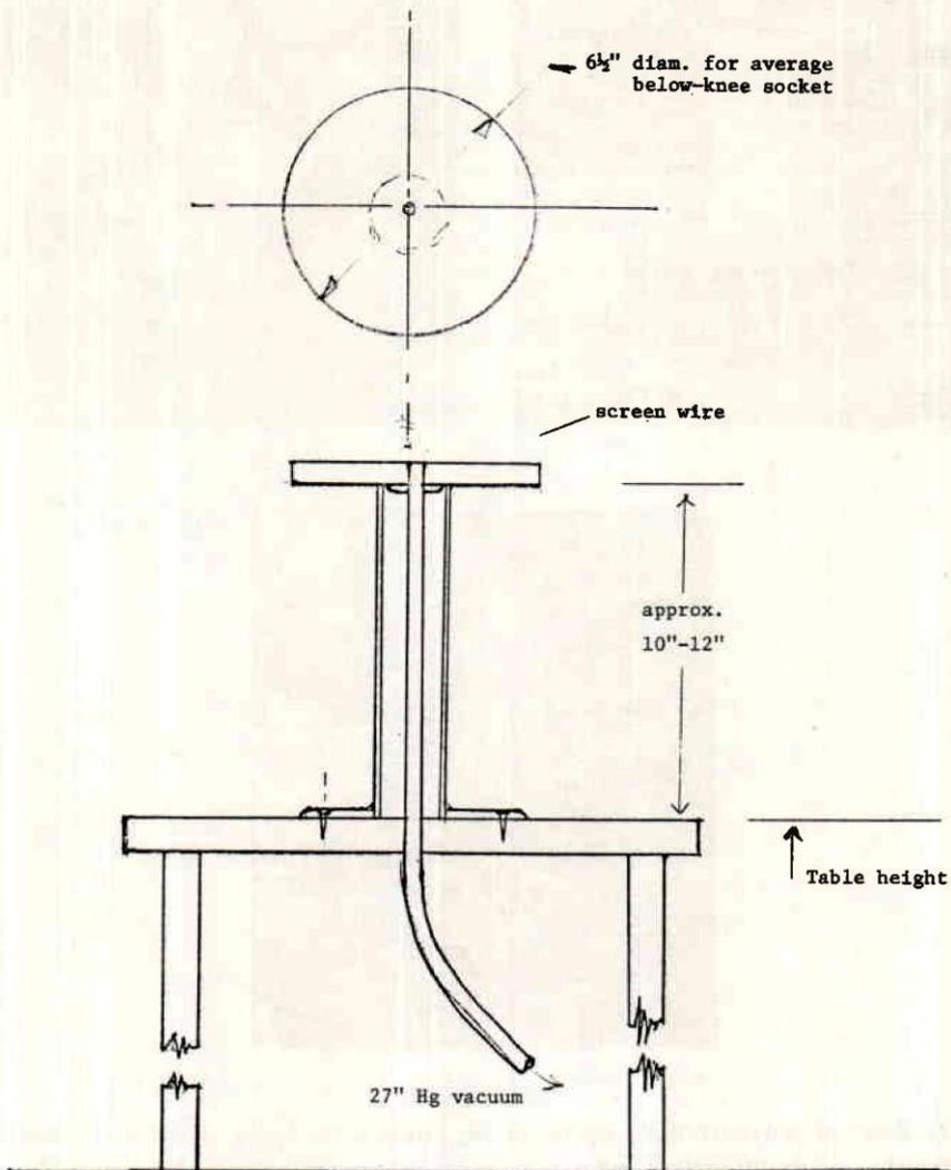
No special equipment is required other than a workstand that will support the male model so that vacuum can be applied during the forming process.
