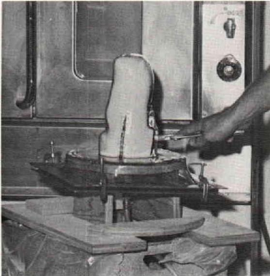
If webs form at the base, use pliers to pinch the sides together so that the inner surface is smooth.
