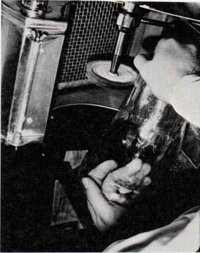
FIGURE 19. —Polishing of poly methyl methacrylate check socket.
