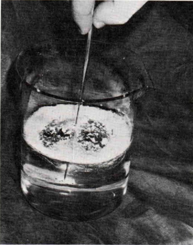
FIGURE 15.—Stirring of catalyst into methyl methacrylate.
