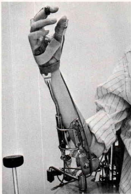
FIGURE 17 —Forearm rotation is caused by a linear pull on the sliding sleeve of pronation-supination unit.
