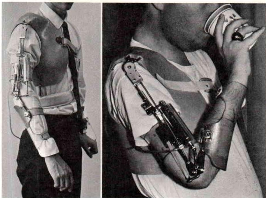
FIGURE 11 (A & B)—Arm brace with CO 2 piston actuator to provide elbow flexion.
