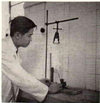
2. Setting up a BE socket in the upper extremity alignment jig.
