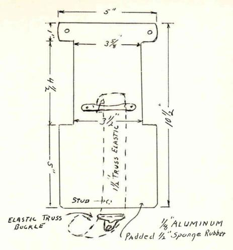
any patient as the weight on the crutch shelf is thrust against the uprights of the crutch, thus minimizing the strain on the wood screws.
