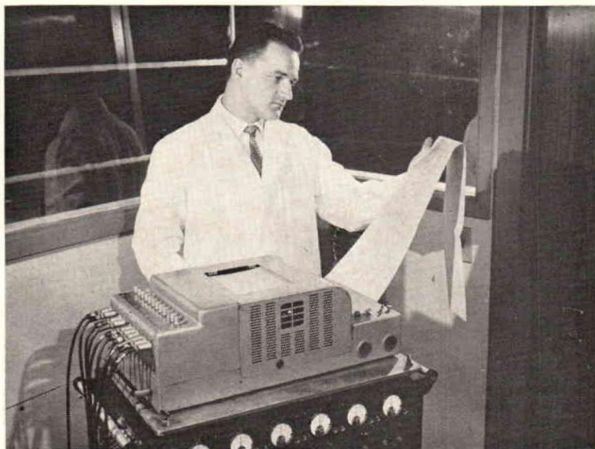
Figure 7. Twelve force plate channels record forces in three planes for each leg during the stance phase of gait. The measures obtained include curves of vertical, horizontal, fore and aft shear, medio-lateral shear and torque forces as well as instantaneous center of pressures on x and y axes.
