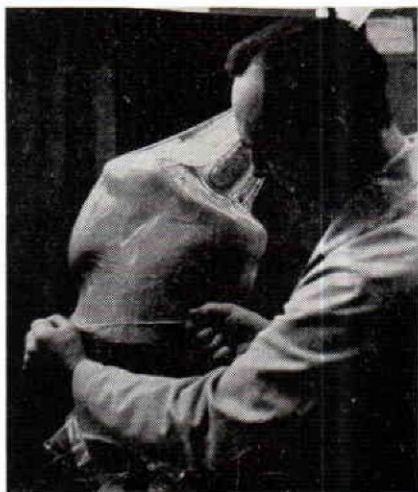
9. Stringing the resin after the vacuum has been applied.
