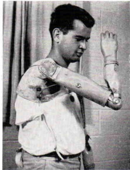
Fig. 6. This shoulder mechanism was designed by Colin A. McLaurin, Northwestern University Prosthetics Research Center. It is a multi-positioned shoulder with a spring detent lock. This mechanism allows a patient with bilateral shoulder disarticulations a greater range of terminal device positioning with positive locking.
