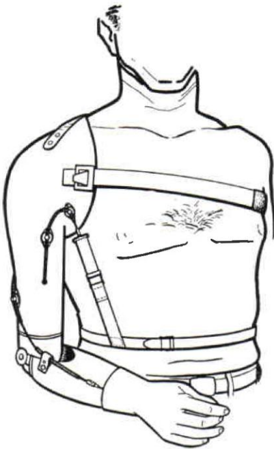
SCAPULAR ABDUCTION DUAL CONTROL WITH SHOULDER ELEVATION ELBOW LOCK
