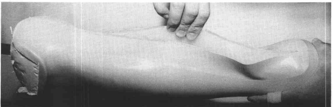
Figure 9. Slit the lamination with a razor vertically to connect the drill holes. The polyethylene panels are used to determine the shape and size of the elastic panels that have been trimmed to size and are to be inserted into the bladder.
