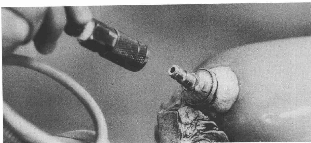
Figure 2. Female couple of air hose to male connector on Cast Off Valve.
