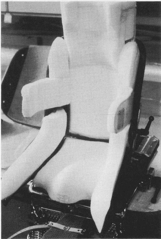
Figure 5. Foam rubber pieces have been glued in place and ground to proper contour and fit.
