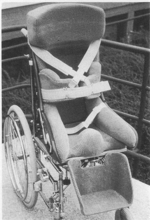
Figure 9. Completed seat showing restraint system and anterior thoracic extension.
