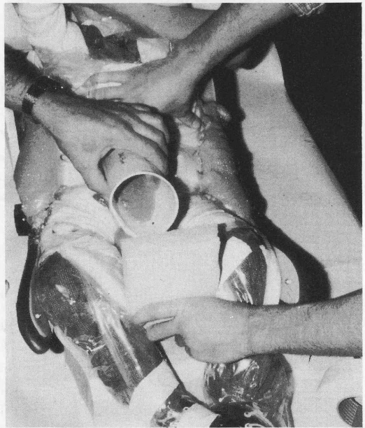
Figure 6. The child is held in place while the void between him and the seat is filled with polyurethane foam. Child is protected against exposure to foam with a layer of plastic film and against thermal burns with a layer of foam rubber. This also allows for the layer of foam rubber to be subsequently added for comfort.
