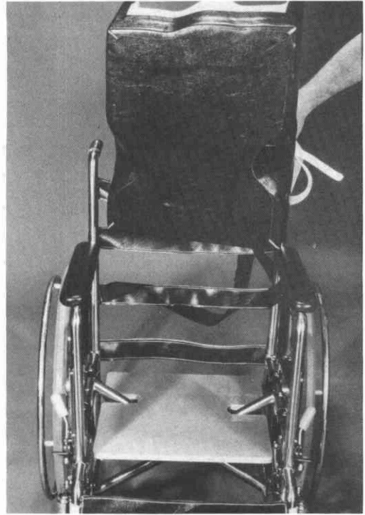
Figure 35. Standard upholstery is removed and replaced with straps so the seat can be recessed down and back between the bars.
