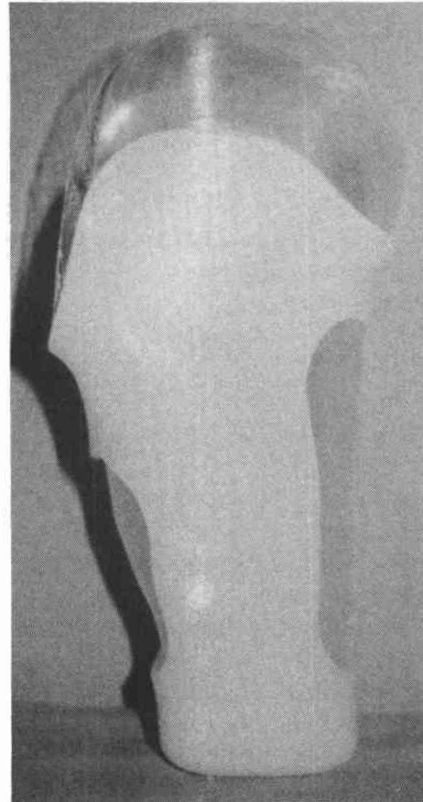
Figure 9. The socket frame and inner socket assembled.
