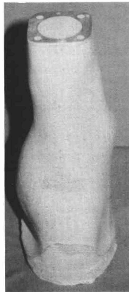
Figure 3. The modified plaster model complete with adaptor, ready for vacuum-forming of the Surlyn® inner socket.
