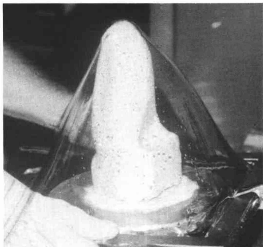
Figure 1. A transparent socket is vacuum-formed over a plaster cast that has been modified in the usual manner.
