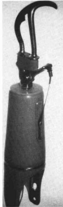
Figure 6. The Prehension Actuator provides powered opening for a variety of conventional hooks. Closing force is controlled by the number of rubber bands applied. (Courtesy of Hosmer Dorrance Corporation.)
