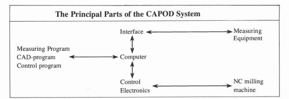
an acronym of Computer Aided Prosthetic and Orthotic Design. The objective of this project is to develop a CAD/CAM system which fulfills the criteria mentioned above. The objectives of the CAPOD system are as follows:
