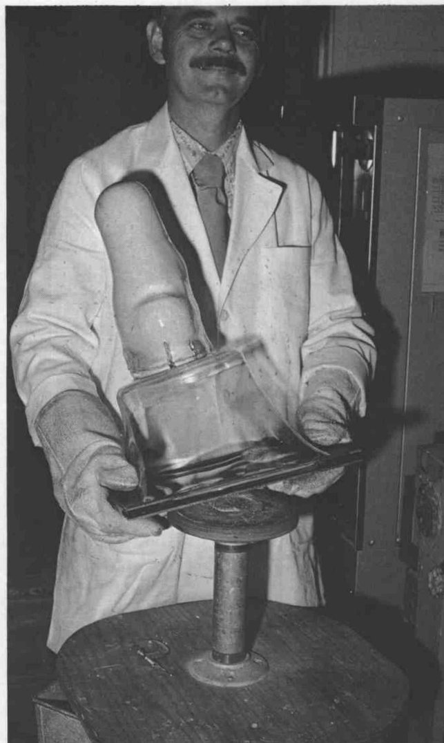
Vacuum-forming a below-knee socket with use of a platen and form for holding plastic sheet.
