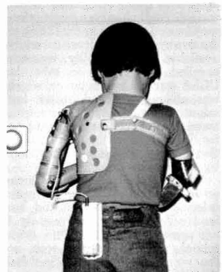
FIG. 3. This youngster with right upper phocomelia and left amelia was given an opposition post early. A standard left shoulder-disarticulation prosthesis provided little function. A hybrid system utilizing an OCCC electric elbow and a Michigan Electric Hook, provides greater function. Both units are powered by one battery pack.
