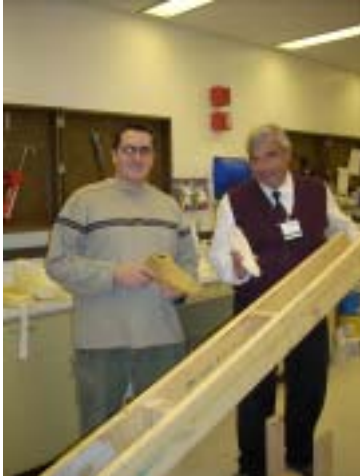
Andrew Hansen, Ph.D. (left), holds a cosmetic cover for a prosthetic foot. Rich Marrano (right), a teacher at Crystal Lake South High School, holds a Shape&Roll Prosthetic Foot core made of copolymer. In the foreground is a lever press that can be used in economically challenged countries. It is easy to assemble and uses economical and accessible materials to create the Shape&Roll Prosthetic Foot.
