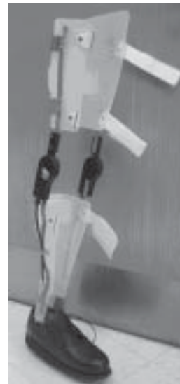
Figure 1: Custom fabricated stance-control KAFO.
