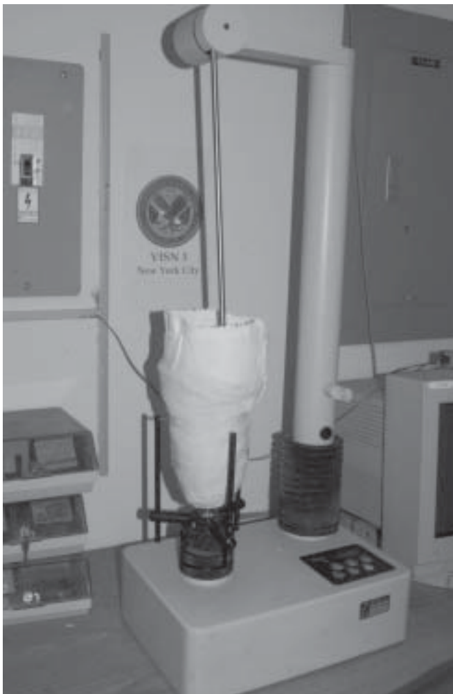
Figure 2: CAD/CAM scanner digitizing a cast of a residual limb.
