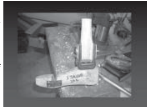
Transtibial prosthetic components built from locally available materials. (Photograph courtesy of E. Pennington-Ridge)
