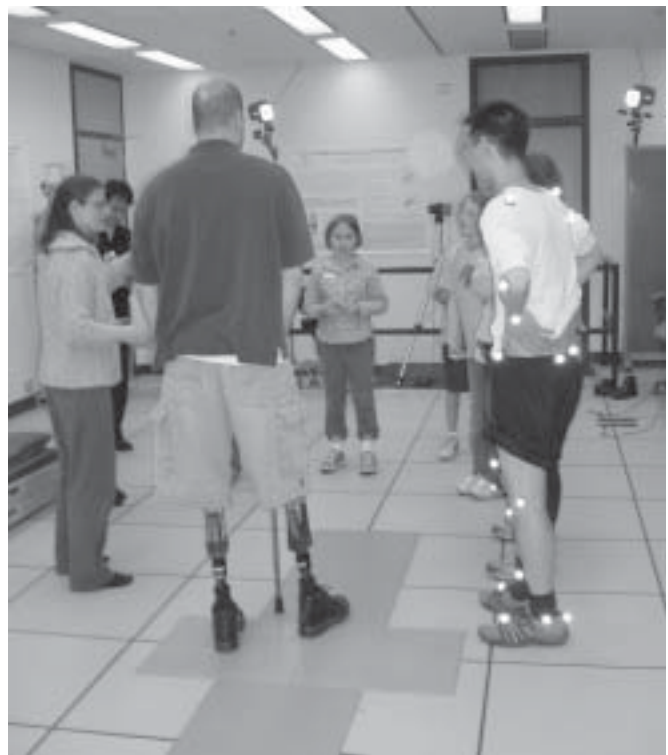
Figure 3: (From left to right) Stefania Fatone, Ph.D., Brian Ruhe, M.S., and Po-Fu Su, M.S., explain and demonstrate motion analysis using force plate and infrared cameras.
