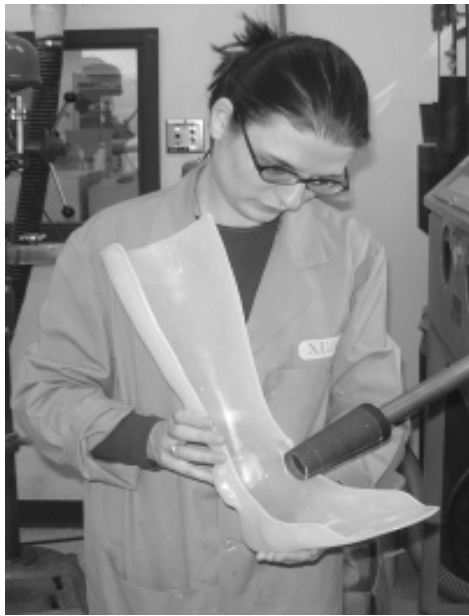
Stefania Fatone works with a router to prepare an orthosis for testing with a subject.
