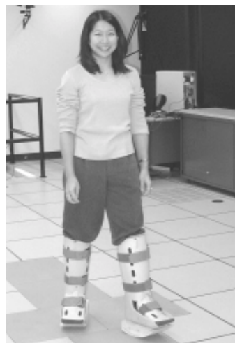
Pinata Hungspreugs demonstrates the rocker feet designed to test hypotheses about gait patterns of persons with lower limb amputations.
