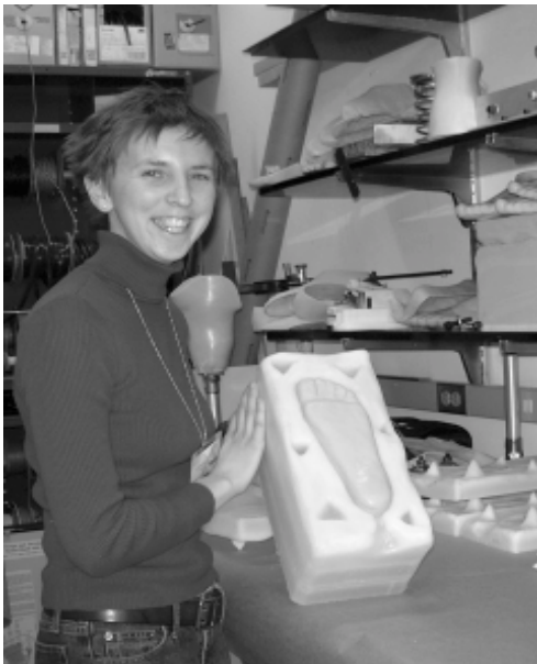
Sophie works with plaster, polyurethane and other materials to create a shell to make the Shape&Roll prosthetic foot more attractive.
