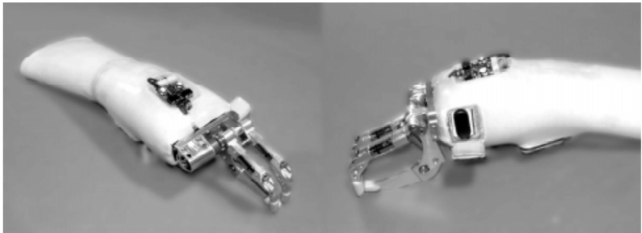
Figure 5: Photographs of new partial hand mechanism and prosthetic interface seen from the right side and a close up of the left. The hand mechanism and associated electronics are mounted on a carbon fiber plate embedded into a silicone-sleeve-socket prototype. In operation, a liner and glove would be pulled over the mechanism and sleeve and the sleeve would be appropriately colored.
