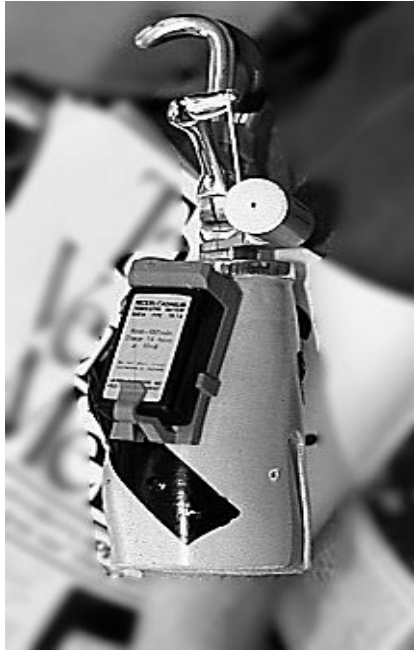
Figure 2: A close up of the original temporary fitting fabricated by our laboratory, showing how the Michigan hook, electronics, and battery were attached to the socket. Single-site myoelectric control was used to control hook opening and closing.
