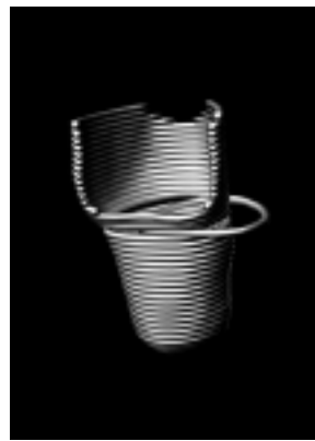
Figure 2: The geometric shape of a limb or socket may be represented as stacked layers where each layer corresponds to a two-dimensional profile.
