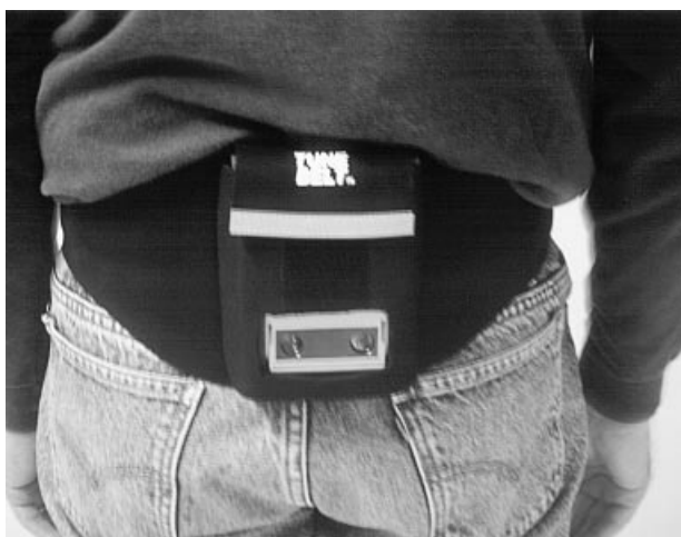
A back pack holds the D.U.R.S. Transponder at approximately sacral level as the subject walks away from the base unit.
