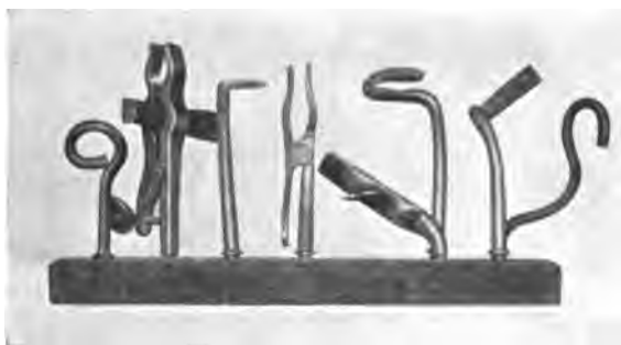
FIG. 161.—The mechanic's tools employed by the patient shown in Fig. 160. These are inserted into the slot at the lower end of the forearm piece and fastened firmly in place by a turn of the screw.
