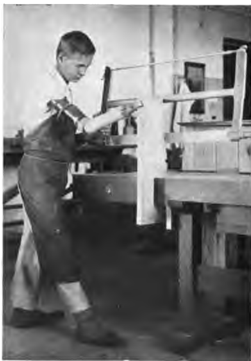
FIG. 151.—The carpenter's apprentice already pictured in the preceding figures, at work with the saw. The artificial limb is used to steady the board.
