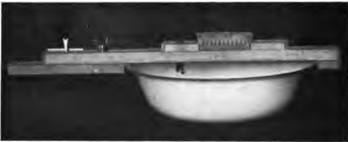
FIG. 167.—A simple toilet arrangement for the one-arm soldier. To permit proper cleansing of the hand, a scrubbing brush and a nail file are fastened firmly to the board which rests on the basin.
