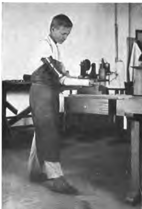
FIG. 150.—The carpenter's apprentice shown in Fig. 149 guiding the plane with his artificial arm.
