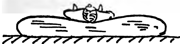
Fig. 6. Person on home-type water bed is supported more by hammocking of cover than by hydrostatic pressure. (JBR 15 Oct 1971)
