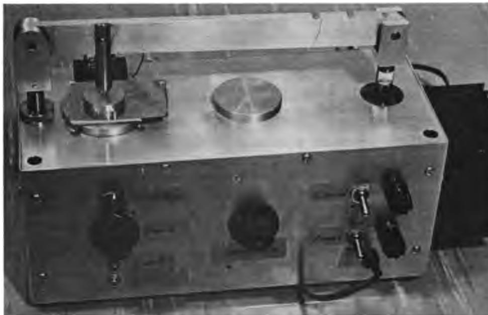
Fig. 2. Servo-controlled platform for testing of static and dynamic properties of elastomers.
