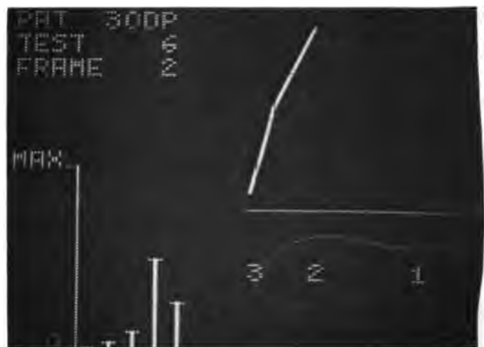
Fig. 3. Leg-foot-pressure display (full scale "maximum" in 40 psi).
