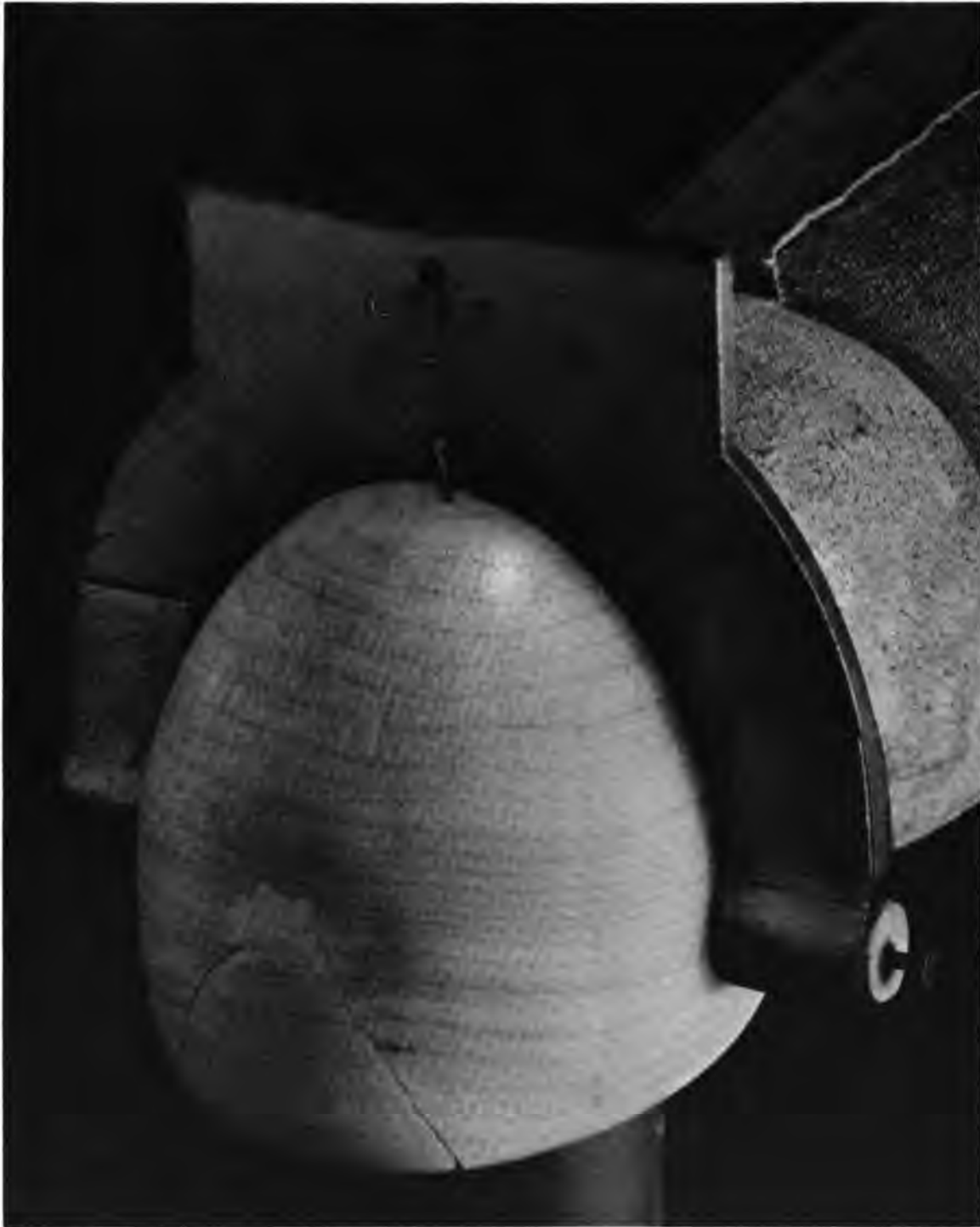
Fig. 2. Using a template to "swing" or contour a wooden knee.
