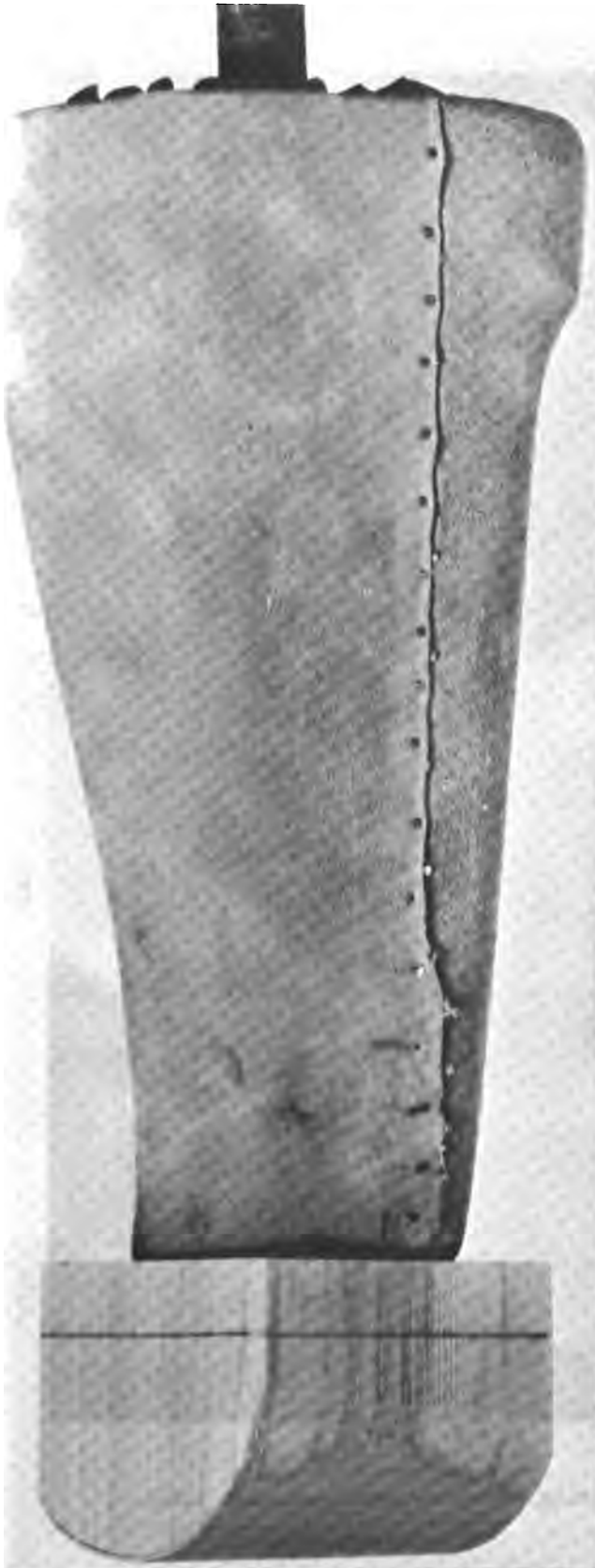
Fig. 1. Inner liner of leather placed over a modified plaster-of-Paris model in the fabrication of a leather socket for thru-knee stump. Here the assembly has been bonded to a willow block that has been rounded in the M-L plane as the first step in shaping it into a spherical knee block. See Figure 2.
