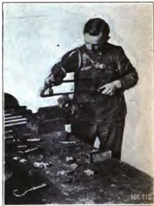
FIG. 143.—Shortened ball connection, with holder for hack saw.
