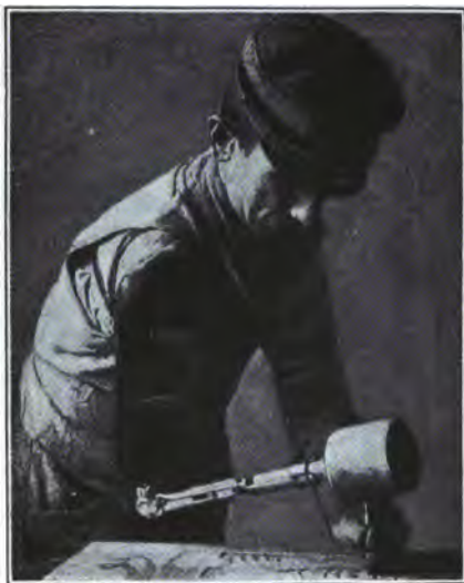
FIG. 103.—Brandenburg work-arm in wood carving. (Radicke.)
