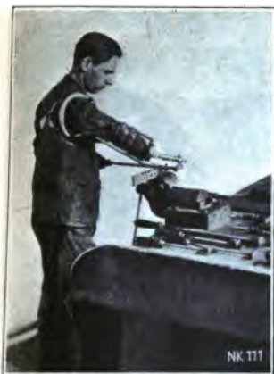
FIG. 138.—Shortened ball connection, with rigid file holder.
