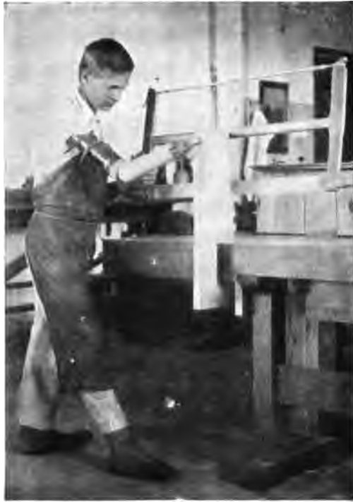
The carpenter's apprentice already pictured in the preceding figure, at work with the saw. The artificial limb is used to steady the board.
