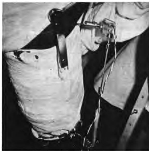
Fig. 6-B. Electrogoniometer measuring motion with patient walking in cast-brace.
