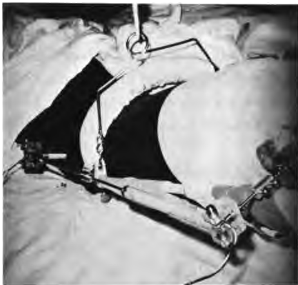
Fig. 6-A. Electrogoniometer measuring fracture motion with patient in traction.
