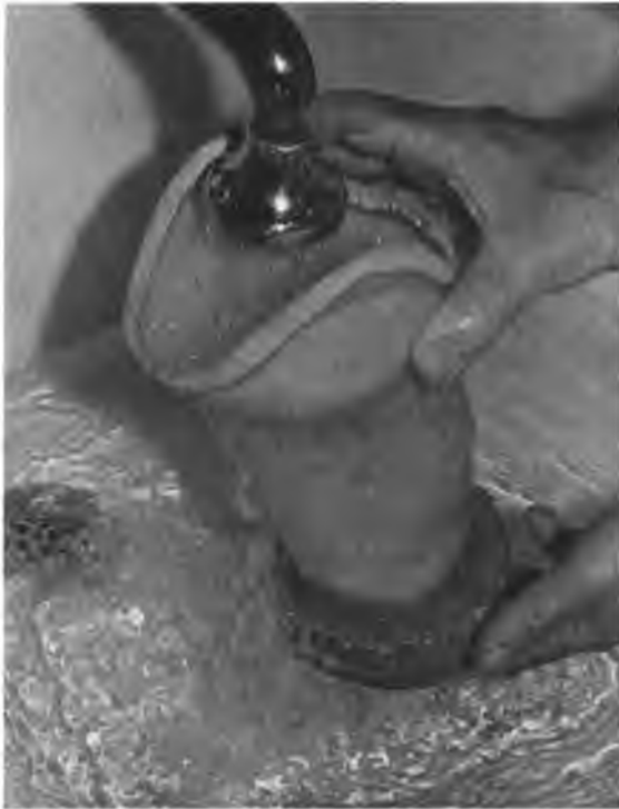
Fig. 4. Demonstration of the porosity of Lightcast socket.
