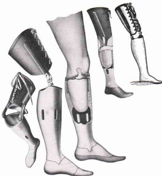
Fig. 9. Some examples of the so-called "conventional" below-knee prosthesis offered by prosthetists for more than a century. Note the sidebars, corset, relatively low brim, and free space at distal end of socket.
