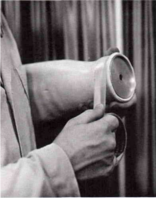
Fig. 12. Socket compressed against turntable with pressure-sensitive tape.
