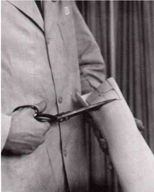
Fig. 3. Cutting out axilla section after tube is heated.
