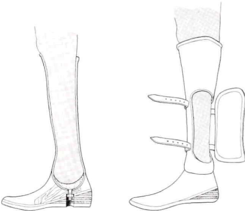
Fig. 6. The prosthesis for a Syme's amputation developed by the Veterans Administration Prosthetics Center.
