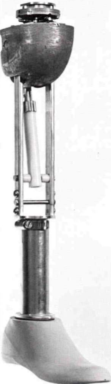
Fig. 11. The Multiplex above-knee pylon-type prosthesis. Various knee-control devices are interchangeable when this unit is used.
