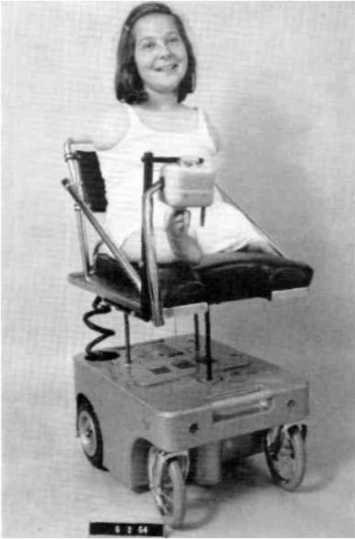
Fig. 9. Battery-powered electrical cart. Speed, direction, and seat height selection are controlled by the amputee by means of joystick arrangement. The cart was developed and constructed at the Child Amputee Prosthetics Project, University of California, Los Angeles.
