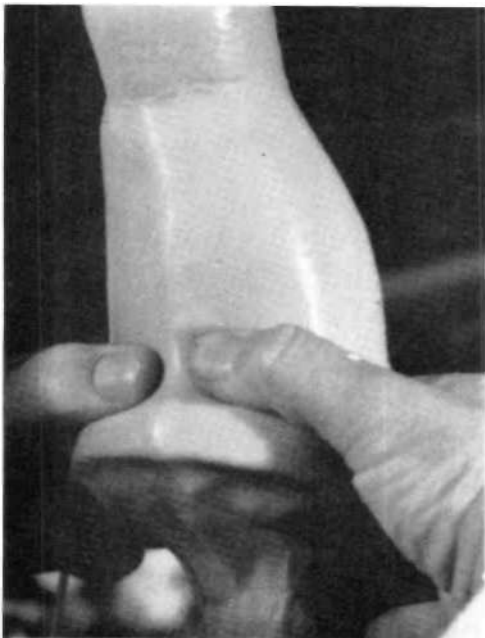
Fig. 42. Working resin into undercut areas.
