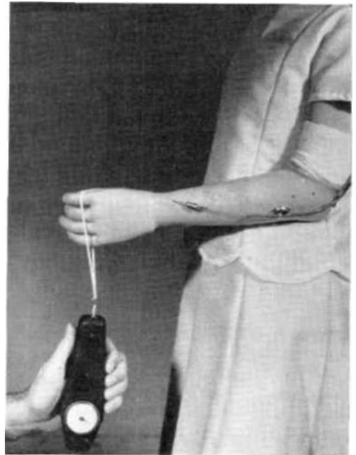
fig. 4. "Live lift"—resisting vertical downward force while maintaining the elbow flexed.
