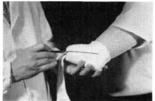
Fig. 25. Drawing a line on the check socket coincident with its long axis.
