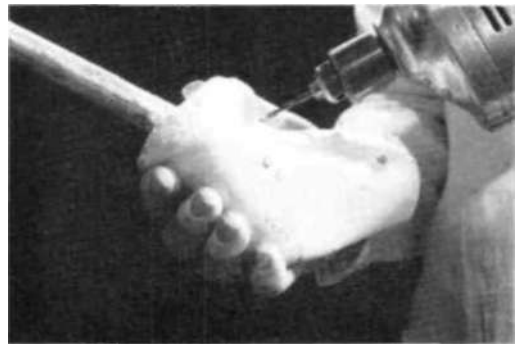
Fig. 40. Drilling 1/8-in. holes through undercut areas at proximal end of the positive model to draw in PVA bag during vacuum lamination.
