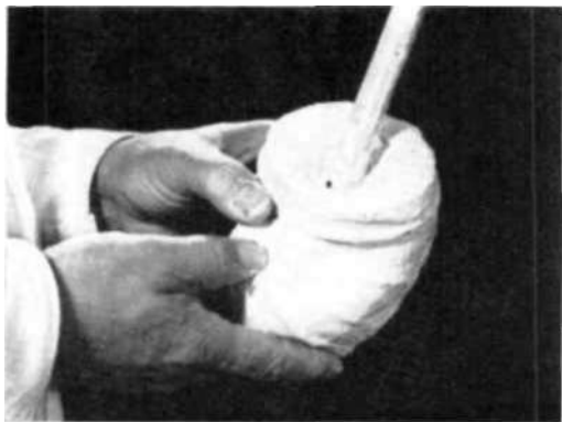
Fig. 34. Check socket filled with liquid plaster of Paris and a hollow pipe inserted into the plaster. The small hole drilled in the pipe will facilitate vacuum lamination.
