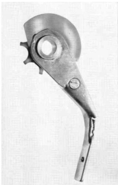
Fig. 5. Typical failure of anchor bar in early clinical study models of the Northwestern University unit.
