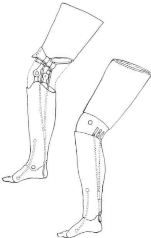
Fig. 6. Anglesea Leg (1800). Below knee at left above knee at right. Knee, ankle, and foot are articulated. From Bigg, H. H., Orthopraxy , 1877.
