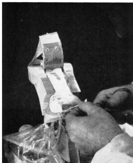
Fig. 50. Fiberglass cloth, used to reinforce keel of SACH foot, being tailored to fit bottom of keel and socket. Note PVA film placed over socket to prevent adherence to fiberglass during laminating process.
