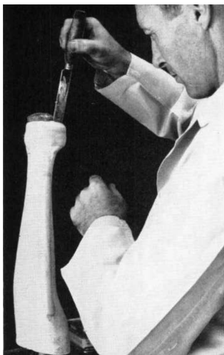
Fig. 47. Placing the spherical washer on the plaster model of the stump so that it may be laminated into the socket. Beeswax is used both to support it in the proper position and to fasten it to the model.
