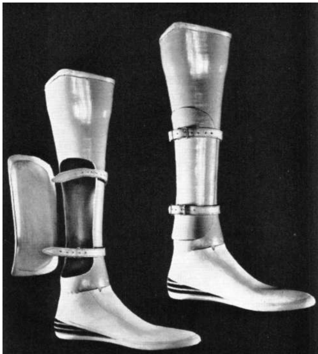
Fig. 10. Syme prosthesis developed by the Veterans Administration Prosthetics Center, New York. The nylon-dacron-polyester socket is provided with an opening in the medial wall. Weight-bearing may be divided, in any proportion, between the proximal rim and the distal portion of the socket.
