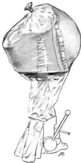
Fig. 17. Truncated PVA cone placed over entire lay-up.
