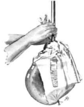
Fig. 18. Resin introduced through the funnels, funnels ready to be removed.
