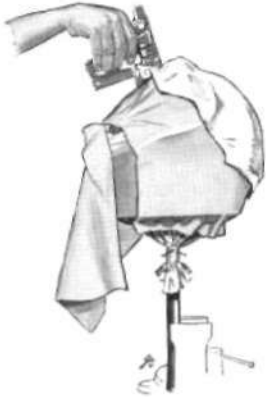
Fig. 12. Glass cloth applied over the stump area.
