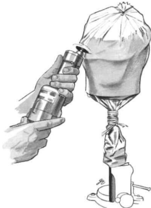
Fig. 21. Cutting the socket free of the mold.
