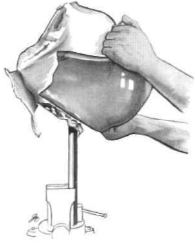
Fig. 22. Removing the socket from the mold.
