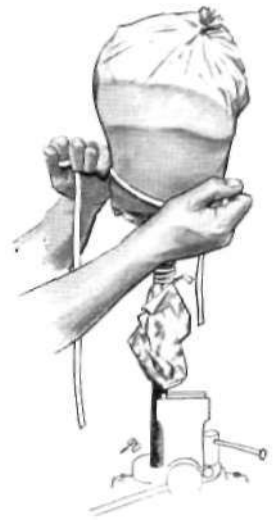
Fig. 19. Saturation of the fabric and removal of air bubbles by "roping."
