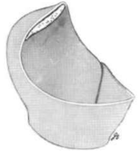
Fig. 23. Finished socket with weight-bearing pad installed.
