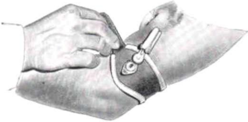
Fig. 15. Placement of the baseplates on the epicondyle strap. They should be so positioned that the cable housings pass through gentle curves from the muscle tunnel to the distal baseplates on the arm socket.
