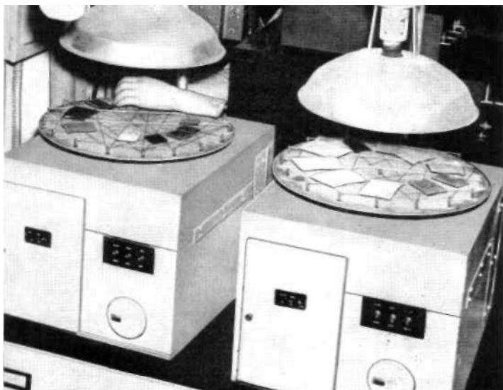
Fig. 5. Apparatus, consisting of ultraviolet lamp and turntable, for determining color fastness of pigments and degradation of plastic materials under exposure to simulated sunlight. Courtesy Army Prosthetics Research Laboratory.
